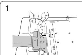
Unfasten the six screws used to secure the stand in place, and then detach the stand from the Display.
